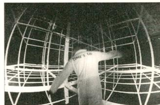
*Over the last few years TIME'S UP has developed a variety of innovative devices, designed to help bridge the gap between virtual and physical environments. Thus SPIN was born - the Spherical Projection Interface. SPIN is a three metre diameter trackball that one walks inside of. As the trackball rotates beneath your feet, the motion is taken over to a virtual space and projections from that space are cast upon the translucent walls of the ball.*
